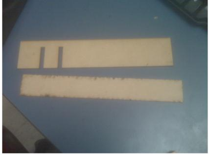
We started by making DWG files for the pedestrians and the vector-etched pieces that will go on top of the sliders. Using ½" MDF, we laser cut the cylinders and tested the fit between the doughnut-shaped radius and the spherical heads. They did not fit on the first try, but they fit after we altered the radius of the inner circle of the doughnut-shaped cylinder. We then glued the three cylinders and sphere together to make the pedestrian, and then glued the pedestrian to its slider.
