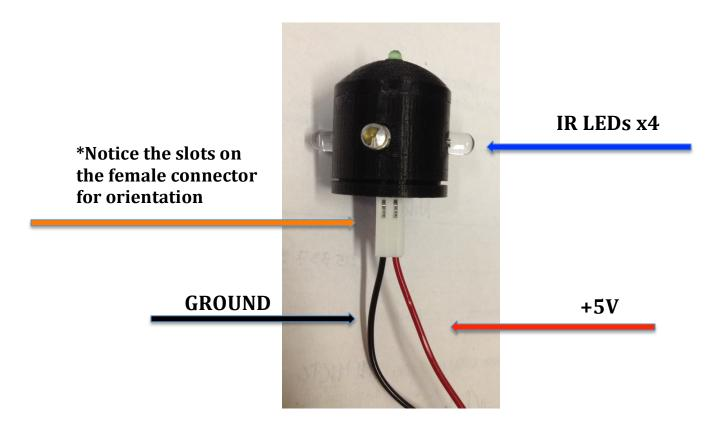
The orientation of your 5V and ground must be correct so as to not destroy our beacons. Your plug must also be solidly attached as to support the weight of the beacon.
